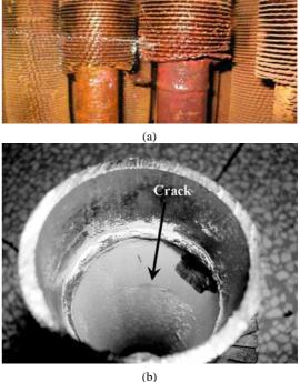
**Fig. 1.** Appearances of the failed tube: (a) leakage location; (b)internal evidence of crack.
