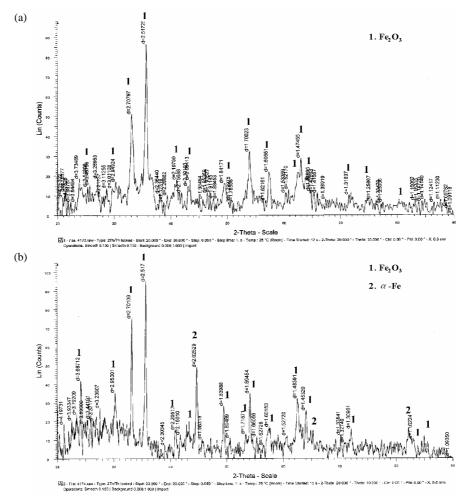
Fig. 4. XRD analyses of corrosion products obtained from different locations of the failed tube: (a) outer surface; and (b) inner surface.
