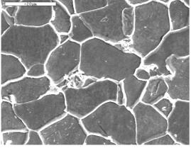
(b) **Fig. 2.** Cross-sectional SEM micrographs of the economizer tubes: (a) new tube; and (b) failed tube.
