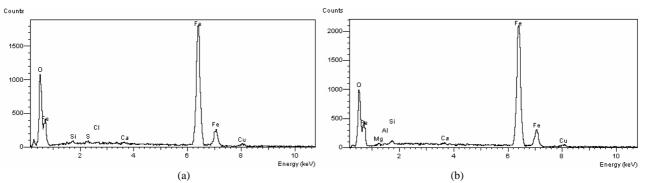
Fig. 3. EDS analyses of corrosion products obtained from different locations of the failed tube: (a) outer surface; and (b) inner surface.
